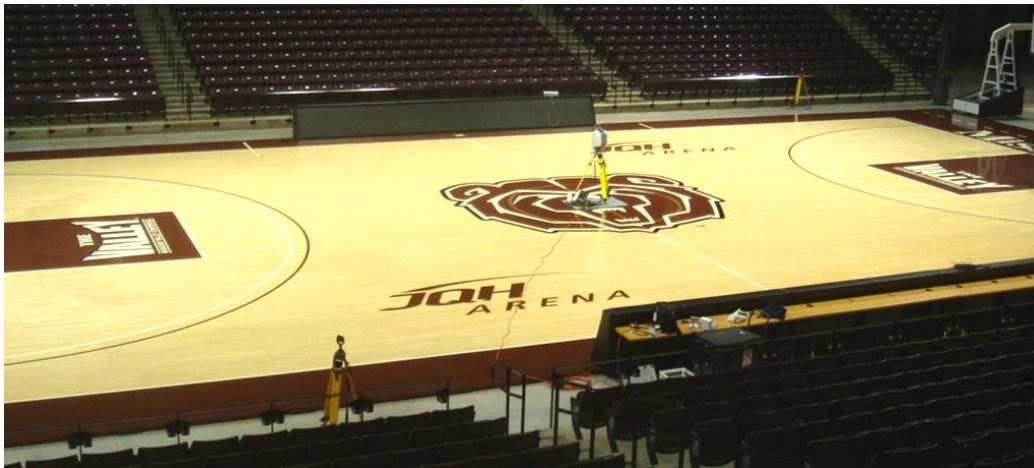
Figure 3. Setup of scanning equipment. The yellow tripods hold the scanner at center court and the targets on each side.
